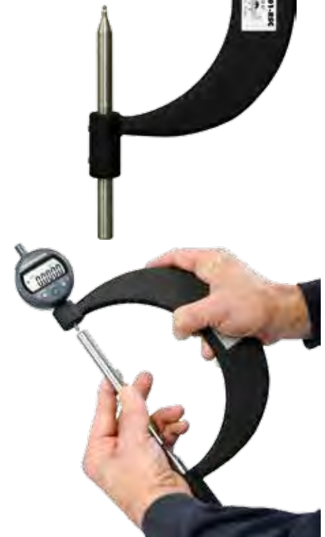
Setting PD-8001-RSC with Rod Standard
